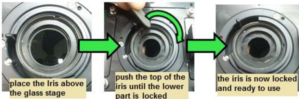
While replacing the iris or cleaning the glass stage, verify that the glass stage is positioned properly in its location: the trimmed edge of the glass stage <sup>1</sup> should be positioned facing the cover<sup>2</sup> as shown on the image below, to avoid dirt and greasy stains, hold the glass stage using the plastic tweezers.
