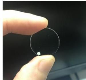
When placing the stage window at its holder, it's very important to make sure that the white rectangle is as shown at the following images (make sure that the white rectangle is at the upper side of the window plate – see below):
