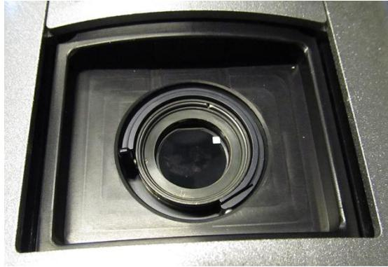
5.2.2.2. Place the tweezers next to the silver pin, at the opposite side of the iris lever, then push the mechanic (not too strong) counter clockwise until it will be released from the silver pin:
