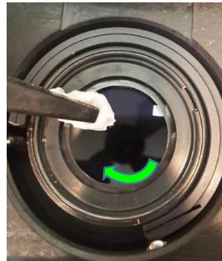
4. To remove fatty materials, immerse the lens cleaning paper in alcohol and repeat step 3 above.
