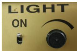
The round knob to the right of the switch controls the intensity of the LED ring.
